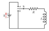
57. In the figure,  $R = 15 \Omega$ , L = 50 H, the ideal battery has  $\varepsilon = 10$  V, and the fuse in the upper branch is an ideal 3.0 A fuse. It has zero resistance as long as the current through it remains less than 3.0 A. If the current reaches 3.0 A, the fuse "blows" and thereafter has infinite resistance. Switch S is closed at time t = 0. When does the fuse blow?
