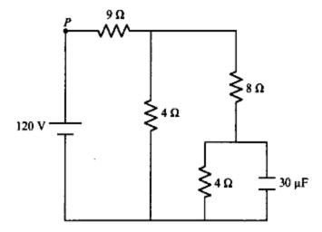
In the circuit shown above, the battery has been connected for a long time so that the currents have steady values. Given these conditions, calculate each of the following.
