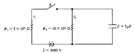
In the circuit shown above,  $i_1$  and  $i_2$  are the currents through resistors  $R_1$  and  $R_2$ , respectively.  $V_1$ ,  $V_2$ , and  $V_c$  are the potential differences across resistor  $R_1$ , resistor  $R_2$ , and capacitor C, respectively. Initially the capacitor is uncharged.
