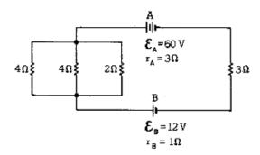
A circuit consists of battery A of emf  $\mathcal{E}_{A}$  = 60 volts and internal resistance  $r_{A}$  = 3 ohms; battery B of emf  $\mathcal{E}_{B}$  = 12 volts and internal resistance  $r_{B}$  = 1 ohm; and four resistors connected as shown in the diagram above.
