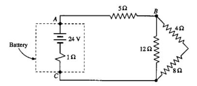
A battery with an emf of 24 volts and an internal resistance of 1 ohm is connected to an external circuit as shown above.
