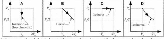
Rank the amount of work that is done by the gas on the environment for the process shown in each case.
