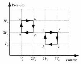
(a) Is work done by the gas for the process  $a \Rightarrow b$  (i) greater than, (ii) less than, or (iii) equal to the work done by the gas for the process  $e \Rightarrow f$ ?
