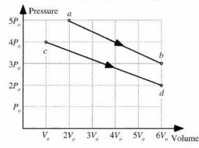
Is the work done by the gas in process  $a \Rightarrow b(a)$  greater than, (b) less than, or (c) the same as the work done by the gas in process  $c \Rightarrow d$ ?
